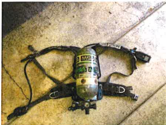
Current SCBA's that were purchased in 2006 and do not meet current standards set forth by the National Fire Protection Agency.
