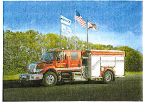
This is an example of the type of fire engine we would replace the current fire engines with. These commercial fire engines are on a standard chassis that are readily available.
